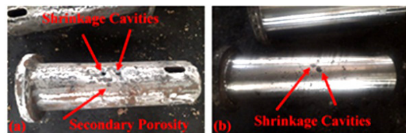
Fig. 2. (a) Casting made by manual method design shown shrinkage adjacent the risers; (b) shrinkage cavities and secondary porosity.
