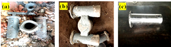
Fig. 5. (a) Two castings with risers and gating system designed by SolidCast; (b) no shrinkage adjacent the riser location; (c) good surface after machining of the casting.
