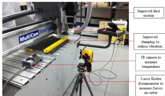
Fig. 3. CNC router used in the machining operation and the cutting set up.
