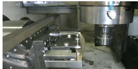
Fig. 10. Finish process of master f-theta lens.
