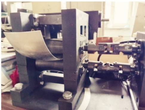
Fig. 11. Forming process of TSRRAR and the experimental device.
