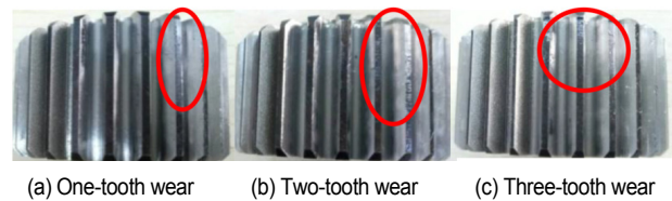
Fig. 5. The wear fault modes of the planetary gear.
