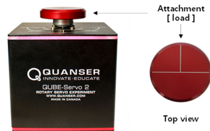
Fig. 3. Actual test platform and removable attachment [Quanser - servo 2].
