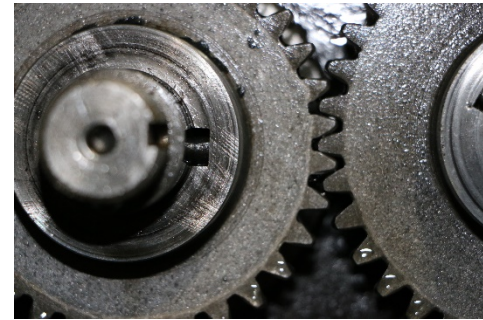
(b) The ordinary spur gear
