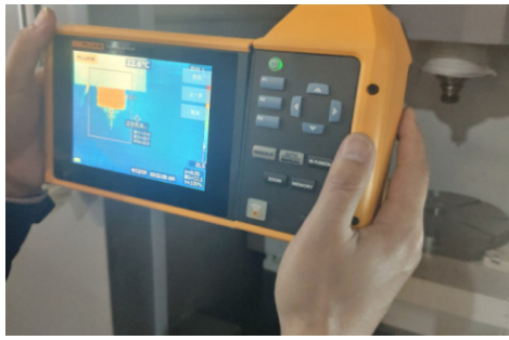
Fig. 4. Spindle temperature measuring with infrared camera.
