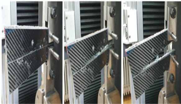
Fig. 6. Experiment process of CFRP-Al foam TDCB specimen for mode 1.
