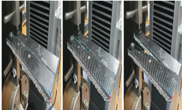
Fig. 12. Experiment process of CFRP-Al foam TDCB specimen for mode 3.
