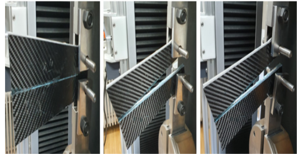
Fig. 4. Experiment process of CFRP-AI6061 TDCB specimen for mode 1.
