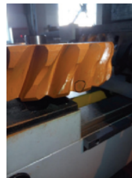
Fig. 15. Meshing contact spots left by the meshing test.
