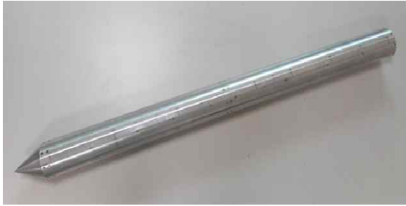
Fig. 1. Shape of the aluminum-alloy missile model possessing high slenderness ratio.
