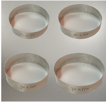
Fig. 8. Test specimens with elliptic section after roll-bending.
