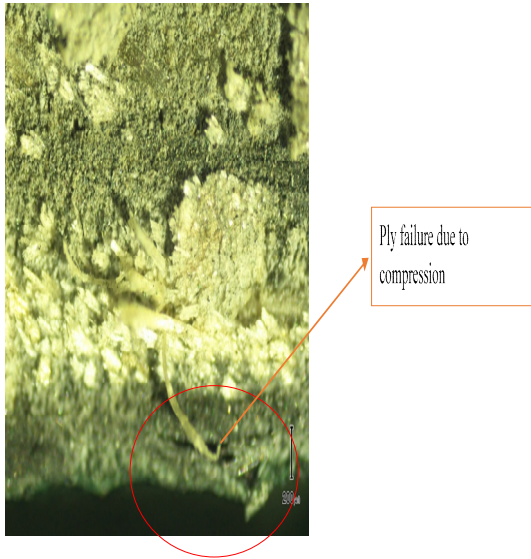
Fig. 18. Ply failure due to compressive load.
