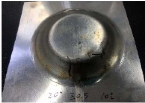
(a) D = 10 mm, S = 200 mm/min, Z = 0.5 mm, T = 20 °C
