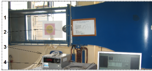
Fig. 1. Setup of the experiment (1. Pitot tube, 2. Hollow wing, 3. Flexible tubes, 4. Digital manometer).
