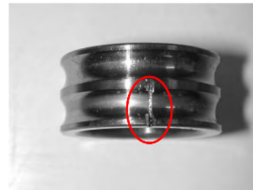
Fig. 25. Inner ring defect.
