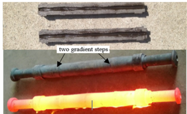
Fig. 12. 1:5 hollow railway shafts after the experiment.
