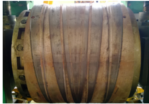
Fig. 11. 1:5 hollow railway shaft rolling mold.
