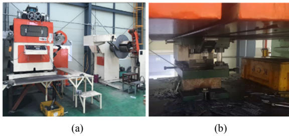
Fig. 6. Device composition for piercing punch durability test: (a) Cutting machine of sheet material; (b) punching press with piercing punch.
