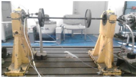
Fig. 6. Physical map of a rotor tester.
