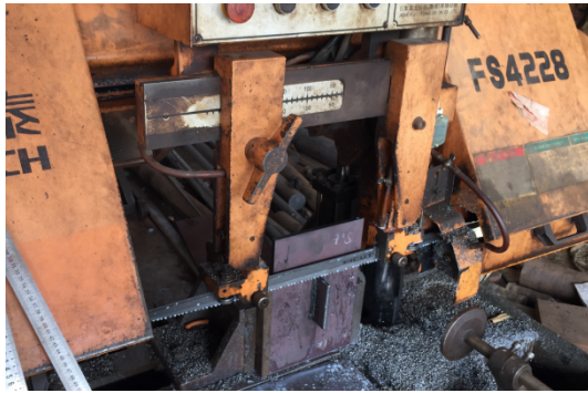
Fig. 7. Experimental set-up of band saw cutting process.
