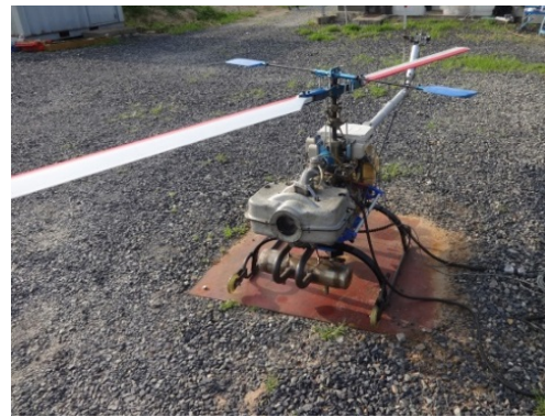
Fig. 2. Freestyle payload measuring system using an agricultural helicopter (AgroHeli-4G) of university's own design.
