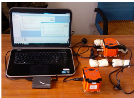
Fig. 9. The composition of vibration testing system.
