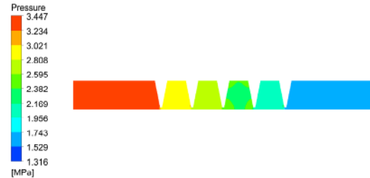
Fig. 7. Static pressure along axial section.
