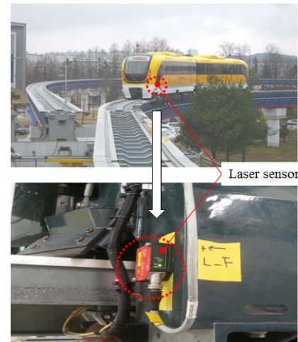
Fig. 19. Sensor locations for measurement of lateral airgaps.
