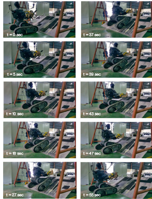
Fig. 10. Time-sequential snapshots of the climbing experiment to verify the performance of the proposed stabilization controller.
