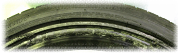
Fig. 9. Real damage situation of a hybrid wheel of fiber angle [\pm 30^\circ] after the impact test.
