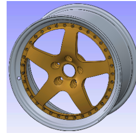
Fig. 2. Hybrid wheel with aluminum alloy disk and composite rim.
