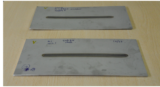
Fig. 7. Concave (upper) and convex deformed shapes (lower) of heat sink welded specimens.
