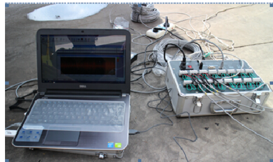
Fig. 12. Measurement system for stresses on the telescopic boom.
