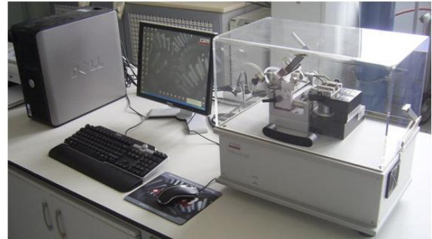
Fig. 10. Wear test module, CSM tribometer.
