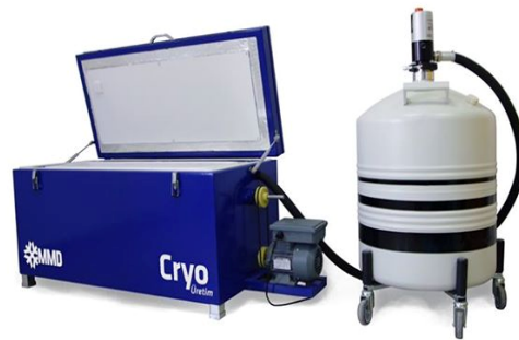
Fig. 1. Cryogenic processing unit.
