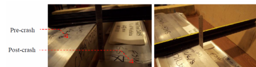
Fig. 9. Bumper deflection measurement method [20].
