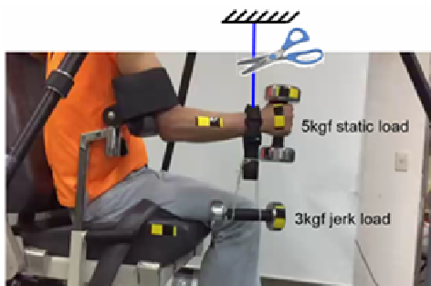
Fig. 1. Test setup for jerk loading at the elbow joint.
