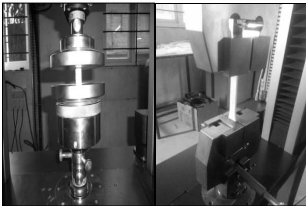
(a) Compression test
