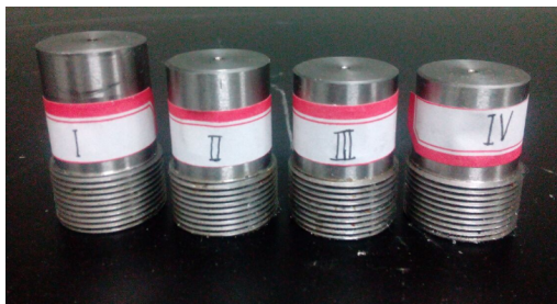
Fig. 3. Photograph of the testing organ-pipe nozzles.
