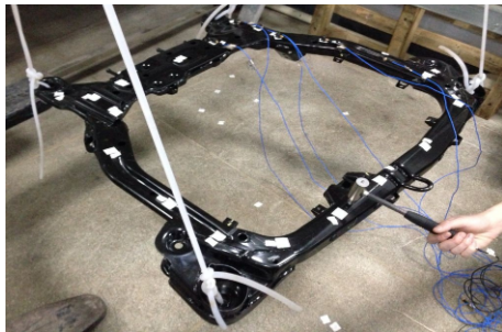
Fig. 2. Modal test of the sub-frame.
