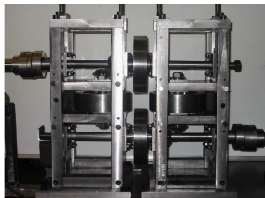
Fig. 2. The test rig for shape rolling.
