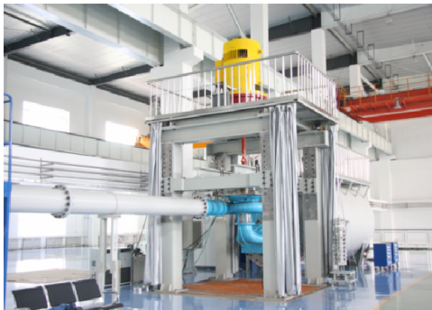
Fig. 4. The investigated pump-turbine model installed in the test rig.
