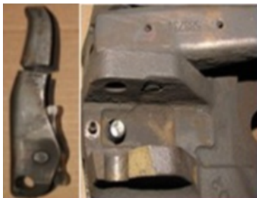
Fig. 3. Damaged PTO finger images.
