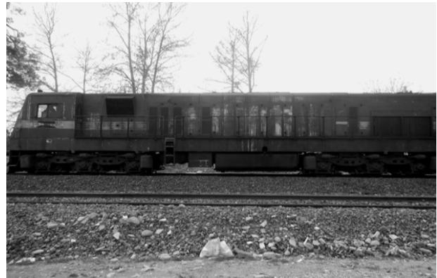
Fig. 2. The locomotive with three axle bogies.
