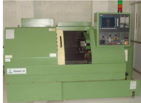
Fig. 2. High speed CNC turning lathe.
