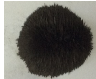
Fig. 8. Mixture of unbonded magnetic abrasives.
