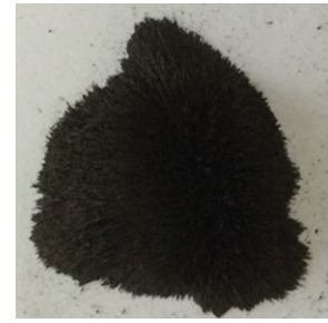
Fig. 6. Mixture of unbonded magnetic abrasives with CNT particles.
