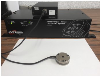
Fig. 8. 6-axis force/torque sensor with a data acquisition system.
