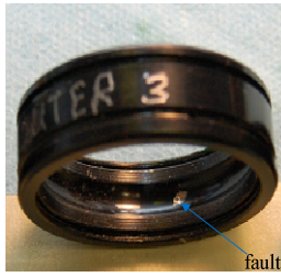
Fig. 11. The defective bearing with an outer race fault.
