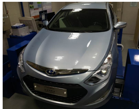
Fig. 15. Photograph of hybrid electric vehicle mounted on chassis dynamometer.
