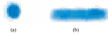
Fig. 6. Brightness distributions of the end-effector point at rest (a); and during motion (b).
