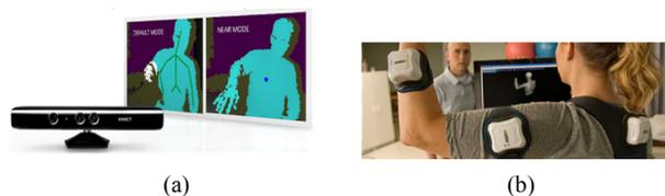
Fig. 1. Existing posture measuring system: (a) Kinect, Microsoft. Motion capture camera using RGB and depth image [9]; (b) K-health, K-vest. A motion sensing module consisting of three accelerometers, three gyros, and three magnetometers [10].
