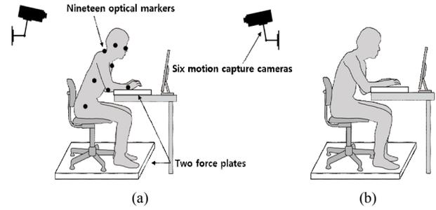
Fig. 3. Experiment setup: (a) two force plates on the desk and under the chair measured the ground reaction force and moment, and 6 motion capture cameras collected the absolute positions of 19 markers on the upper body; (b) the subjects performed the same tasks under 2 posture condition: straight posture and bent posture. Figures a and b show the straight and bent postures.
