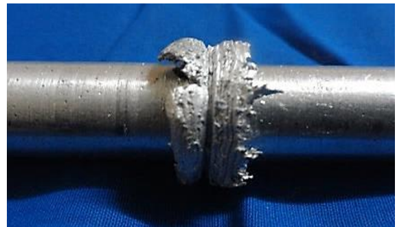
Fig. 7. Joint formed with optimal parameter setting (frictional pressure: 60 MPa, upset pressure: 100 MPa, burn off length: 2 mm and rotational speed: 1500 rpm).
