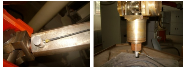
Fig. 10. The disposal position of sensors on parallel manipulator.
