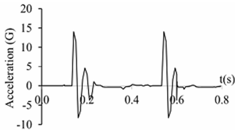
(b) Acceleration of the table along the Z-axis for the dual-impact stroke
