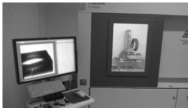
Fig. 8. Examination of the surrounding rock on the micron X-ray computerized tomography system.
