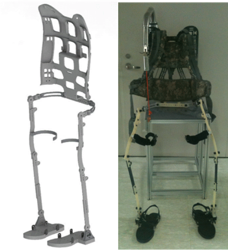
Fig. 1. Prototype of the lower extremity exoskeleton used for human motion analysis.
